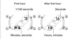
3. Press (A) to reset the measurement time to all zeros.
